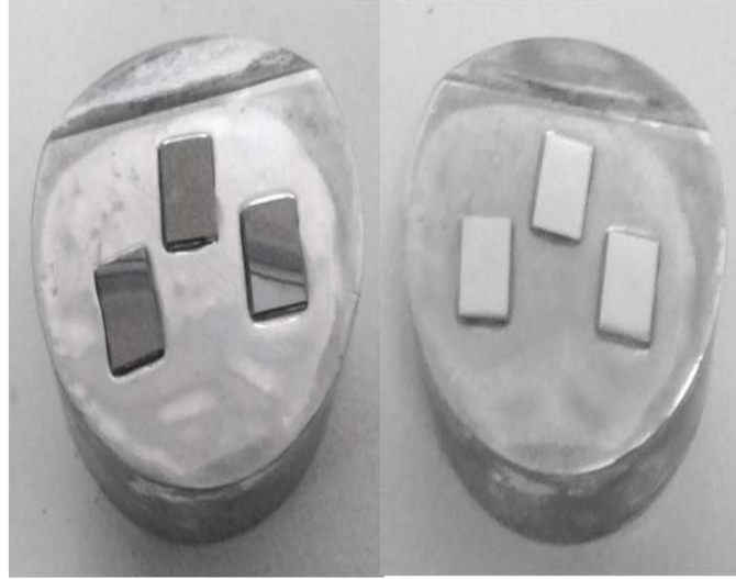
Figure 10. Both pictures show samples mounted in wax on the Buehler cylindrical attachment. The SiO 2 side is facing up. The left picture is samples before polishing and the right is after. The SiO 2 is removed when the dull rainbow is removed.
